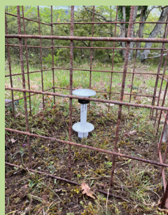
Data logger with protection from wild boars
