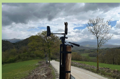
Data logger with protection from wild boars
